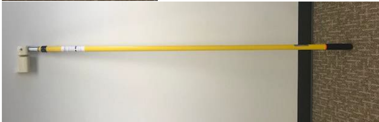
Sample (extension) pole carriage where sample bottle could be affixed using reusable cable ties or elastic bands.
